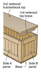
with the vertical grain exposed. Nail each 2x2 with 8d nails every 6 inches, spaced as shown below.
