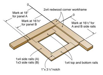
**Side rails** Trim four 1x4s and four 1x3s to  $16\frac{1}{2}$  inches. Along the length at each end, mark and cut  $90^{\circ}$  notches,  $1x3\frac{1}{2}$  inches.
