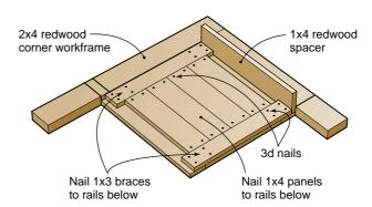
**Paneling** Measure and cut four 1x4s to fit flush between braces as shown for all panels. The boards should overlap rails by at least 1 inch on all sides.
