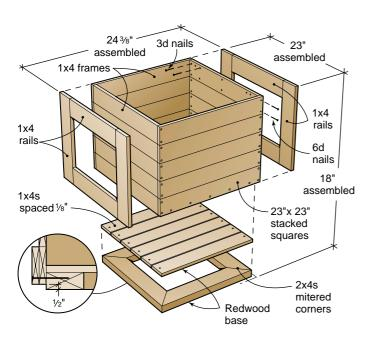
**3. Base** Miter or butt join four 2x4s to form a 215%-inch square base to fit inside the planter. Assemble with one 10d nail per corner. Cut six 1x4s to 21 inches and nail them to the 2x4 base, spaced 1/8 inch apart. Use one 6d nail at each board end. Insert assembled base into planter bottom and attach in the same way as described previously for the Vertical Paneled Planter base.
