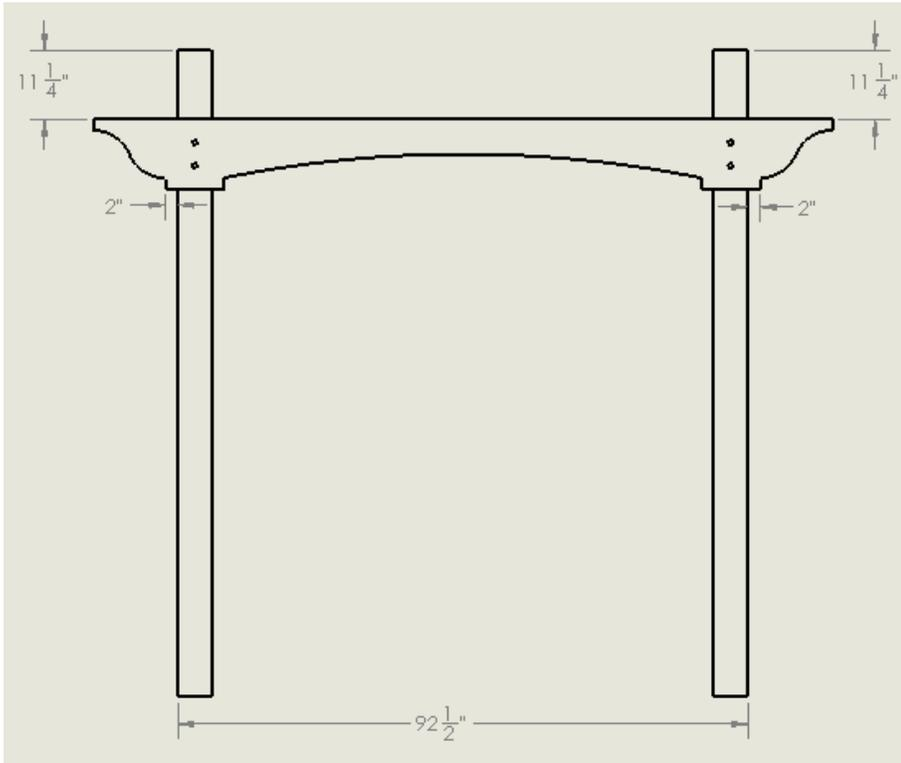
Assemble two 3x12 Bottom Headers on both sides of post using provided hardware
