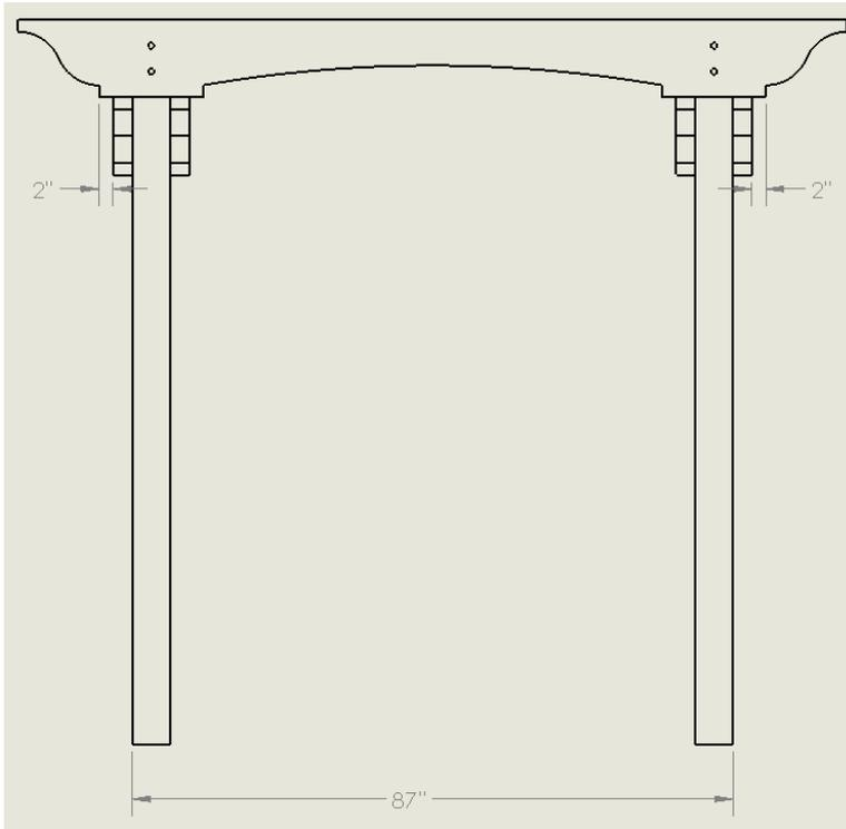
Assemble two 3x12 Top Headers on both sides of post using provided hardware
