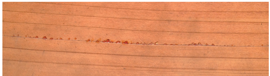
Fig. 1 Small, sticky globules of pitch may bleed to the surface along the grain of properly manufactured and dried redwood.
